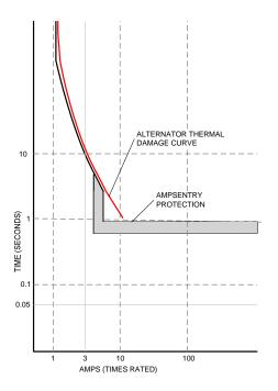
**Short circuit shutdown (51)** -Output current on any phase is more than 175% of rating at time of shutdown. The control replicates the function of a 51V relay by discriminating between short circuit conditions and shutdown conditions, and shutting down the genset as fast as is necessary on a short circuit condition while operating as long as is possible on an overload condition. Control includes algorithms to protect alternator from repeated over current conditions over a short time.
