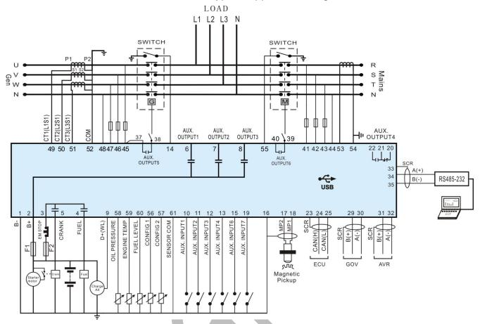
Note: Fuse F1: min. 2A; max. 20A. Fuse F2: max. 32A. Users should select suitable fuse depend on practical application.
